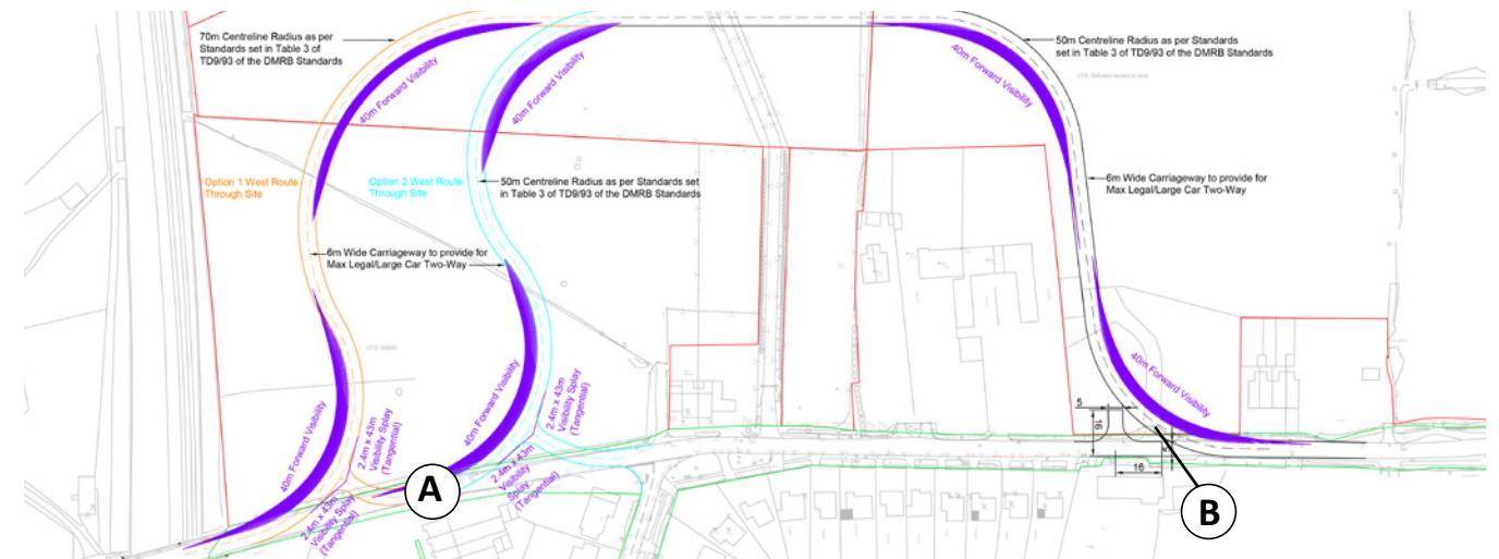
**B** OPTION B: Plan extract illustrating potential access configuration onto Rising Lane.
