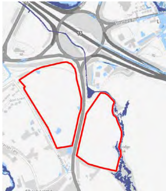
EA Risk of Surface Water Flooding Map
